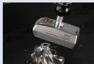
The flying spot type is capable of scanning difficult parts, such as this impeller, precisely and achieves highest scanning accuracy in the class.
